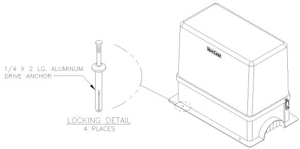
\*Note the receptacles and the concrete slab should be prepared and fully cured before the enclosure is unpackaged.
